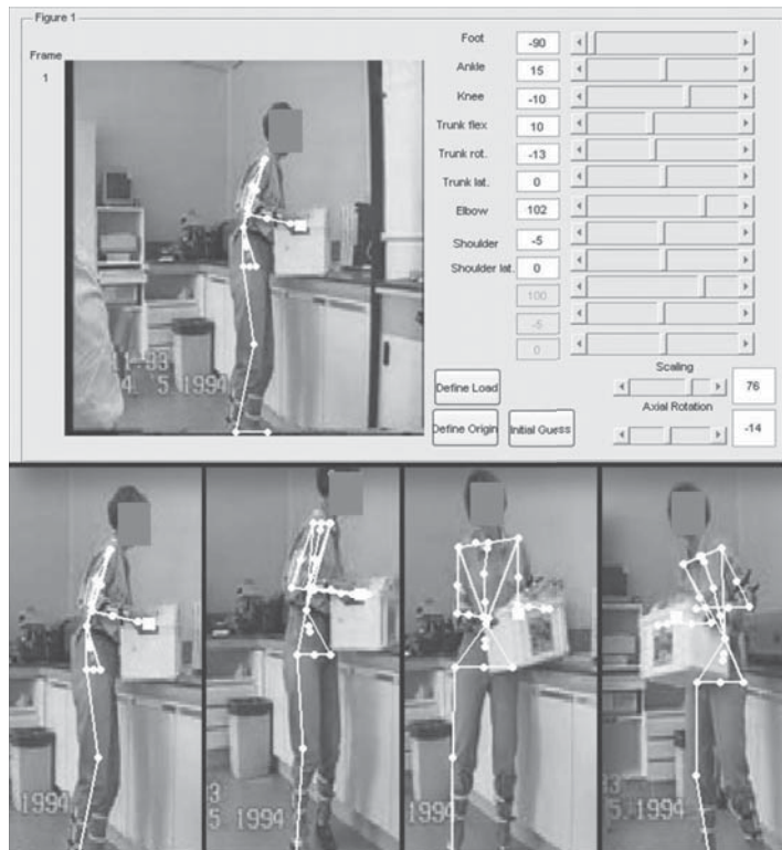
Figure 7.1 | Video analysis method. The graphical user interface depicting a three-dimensional manikin plotted onto a video frame is shown (upper part of the figure). In the lower part of the figure, a typical example of four key video frames of a field-based lifting task is shown that was analyzed by one of the observers.
