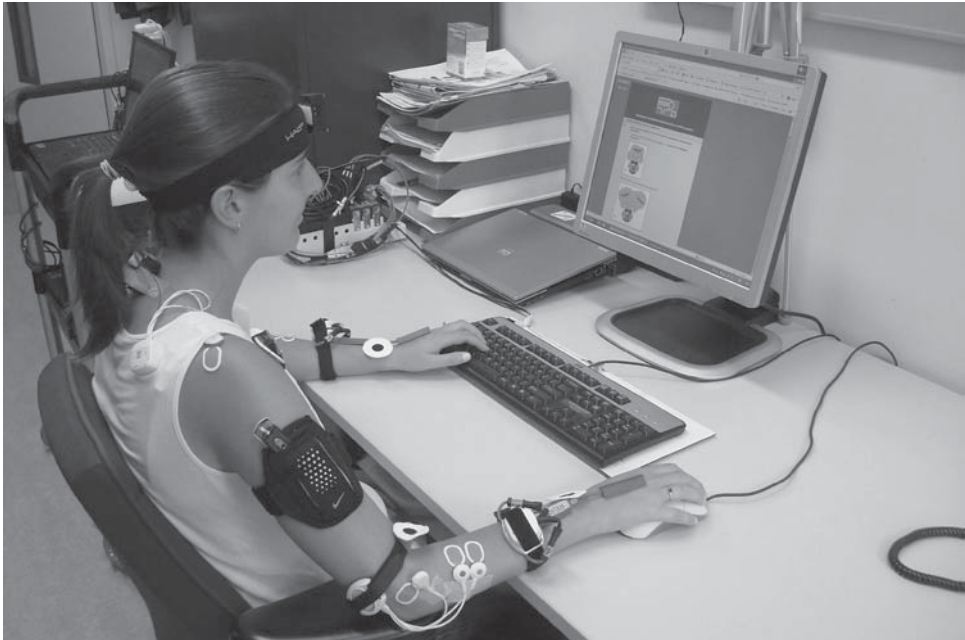
Figure 1. Instrumentation set up on a participant at her workstation. The systems used to measure the biomechanical exposures were chosen to be unobtrusive and allow the participant to perform her regular work without interruption or restriction. Participants were able to move freely at their workstation and to leave the workstation without restraint.
